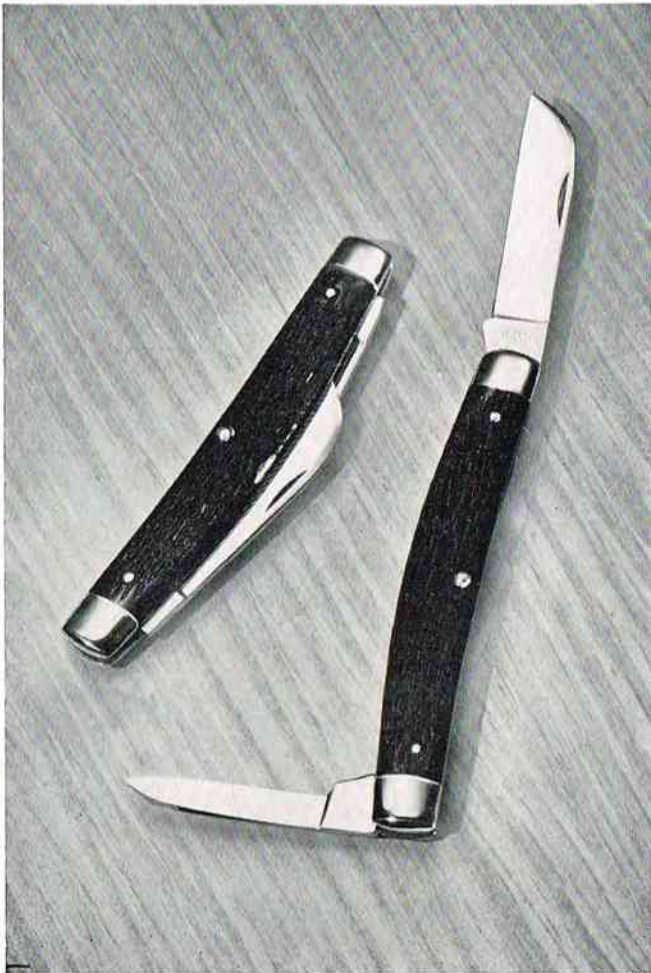
No. 15 Congress Pattern — Two blade pocket knife. Genuine bone stag handle. Nickel Silver double bolsters, brass linings. One 2-inch sheepsfoot blade with 1\frac{3}{4} -inch cutting edge and one 1\frac{1}{16} -inch pen blade with 1\frac{3}{8} -inch cutting edge. 3\frac{1}{2} inches long when closed. Always a leading number.
