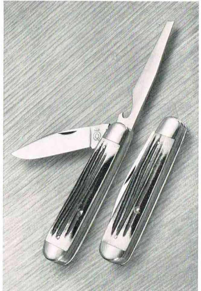
No. 40 Heavy Duty Screwdriver Knife. — Genuine Frontier bone stag handle. Nickel Silver double bolsters, brass linings. Clip blade 2\frac{1}{16} inches long with 2\frac{3}{8} -inch cutting edge and screw driver bottle opener blade 2\frac{3}{4} inches long. 3\frac{1}{16} inches overall when closed.
