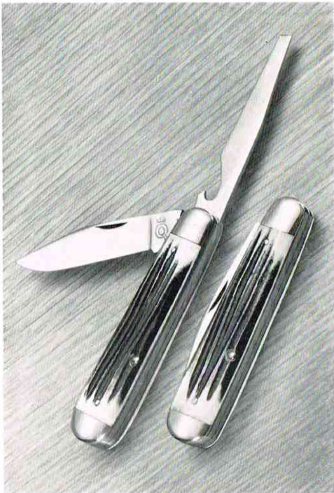
No. 40 Heavy Duty Screwdriver Knife. — Genuine Frontier bone stag handle. Nickel Silver double bolsters, brass linings. Clip blade 2\frac{1}{8} inches long with \frac{2}{8} -inch cutting edge and screw driver bottle opener blade 2\frac{3}{4} inches long. 3\frac{1}{8} inches overall when closed.
